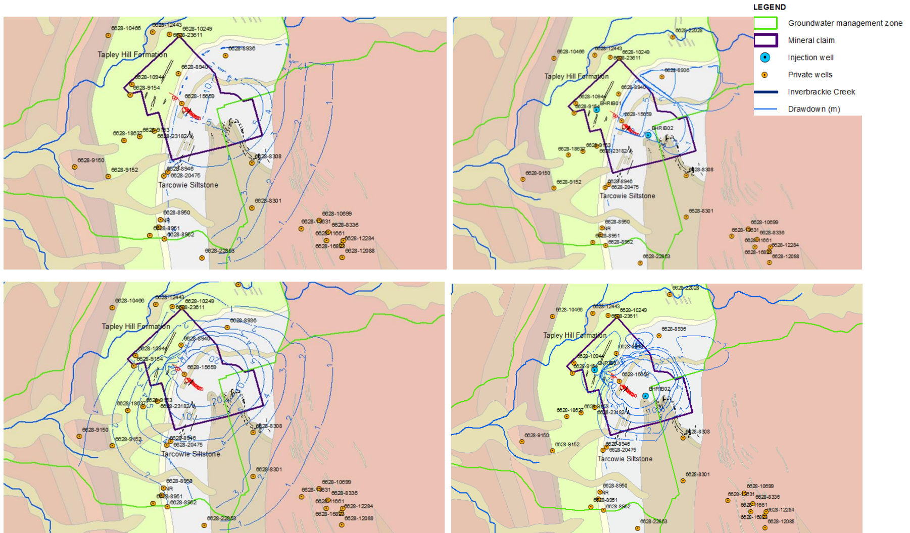
FIGURE 10-23 | DRAWDOWN CONTOUR RANGE ACROSS MINING SCENARIOS AT MINING YEAR 5.5 (TARCOWIE SILESTONE AND TAPLEY HILL FORMATION)
