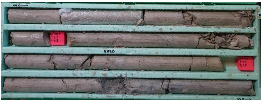
FIGURE 10-7 | EXAMPLE OF THE INTENSE CLAY ALTERATION WITHIN THE SUPERGENE SULPHIDE BLANKET
