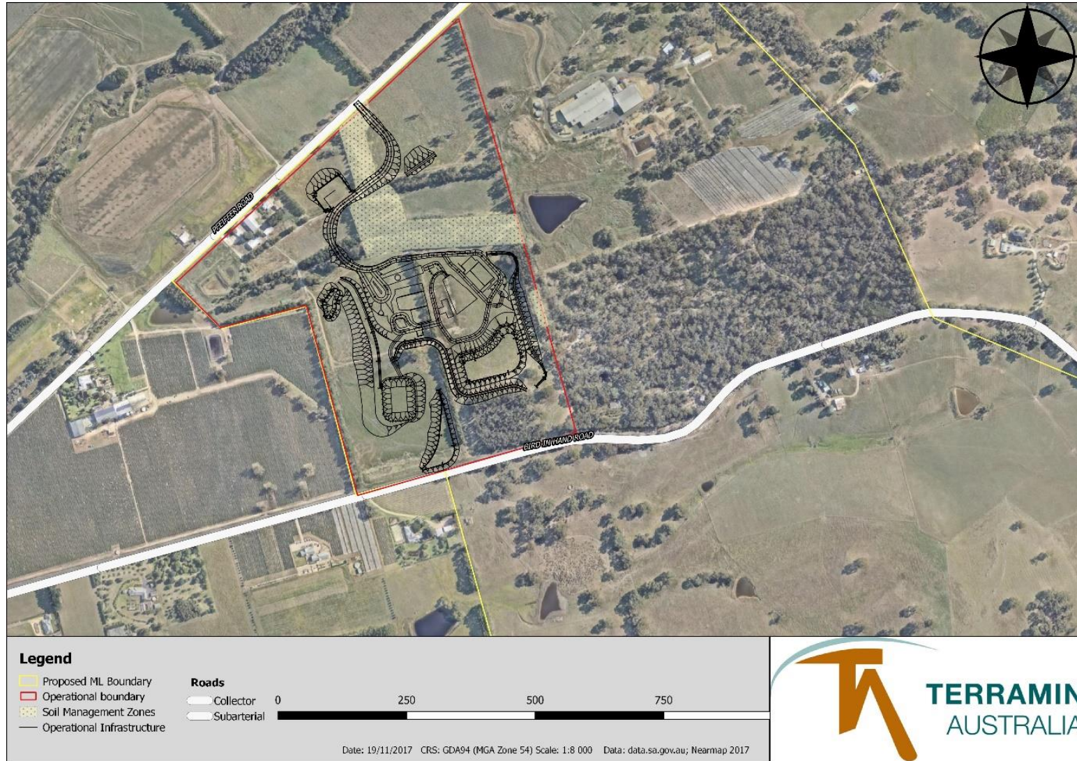
FIGURE 14-23 | IDENTIFIED SITE DESIGN AND SOIL MANAGEMENT ZONES
