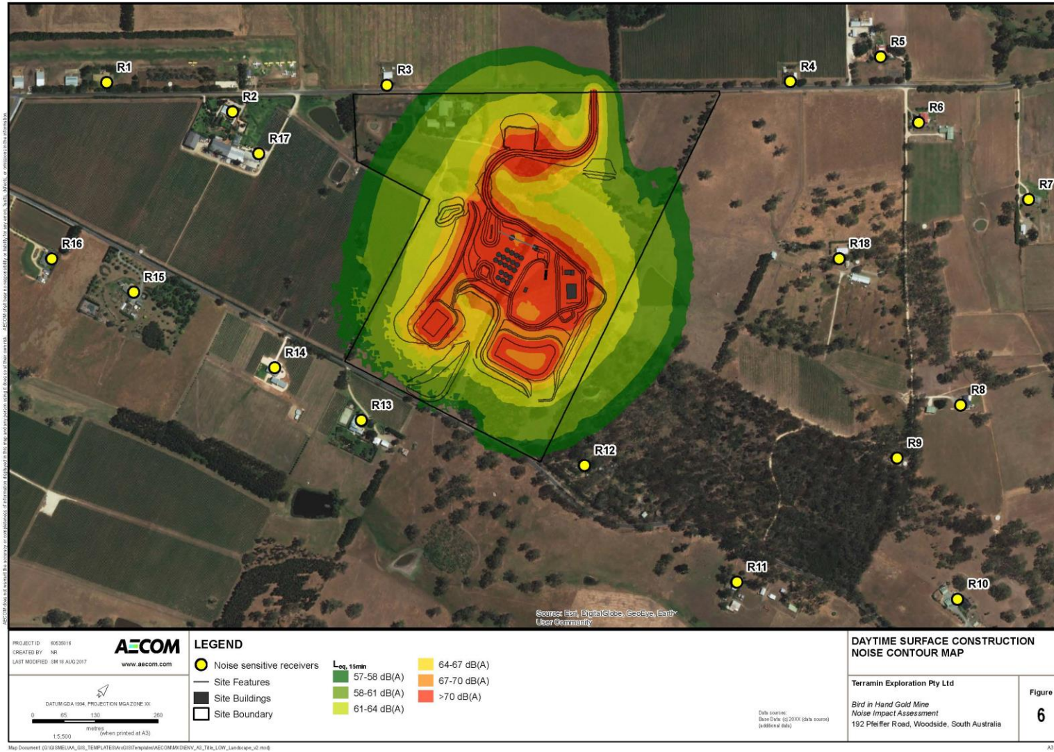
FIGURE 16-4 | DAYTIME SURFACE CONSTRUCTION NOISE CONTOUR MAP
