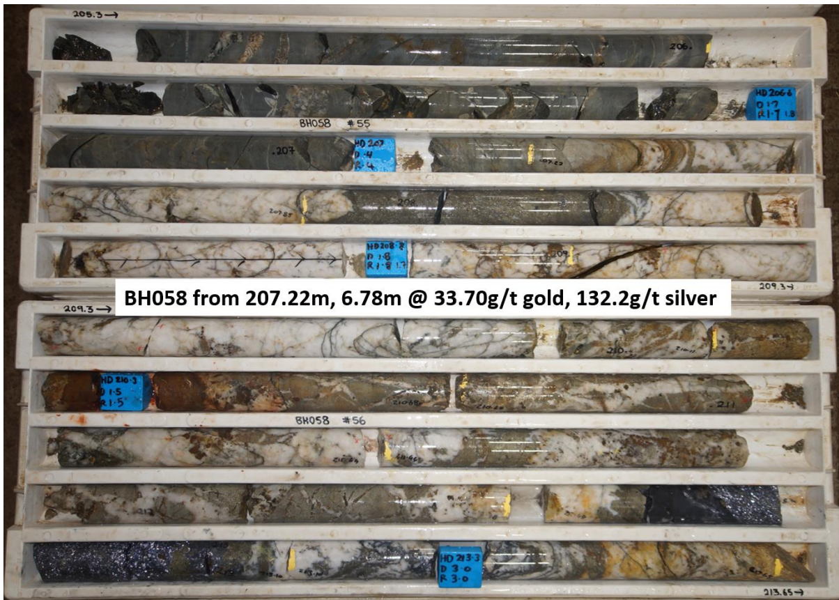
FIGURE 2-31 | INTERSECTION OF RED REEF INBH058, FROM 207.22M, 6.78M @ 33.70G/T GOLD AND 132.2G/T SILVER WEATHERING
