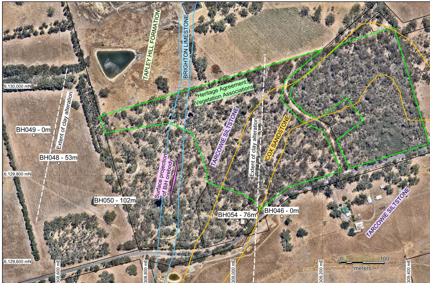
FIGURE 2-32 | DRILLHOLES USED AS EXAMPLES, LABELLED WITH DEPTH OF CLAY DEVELOPMENT
