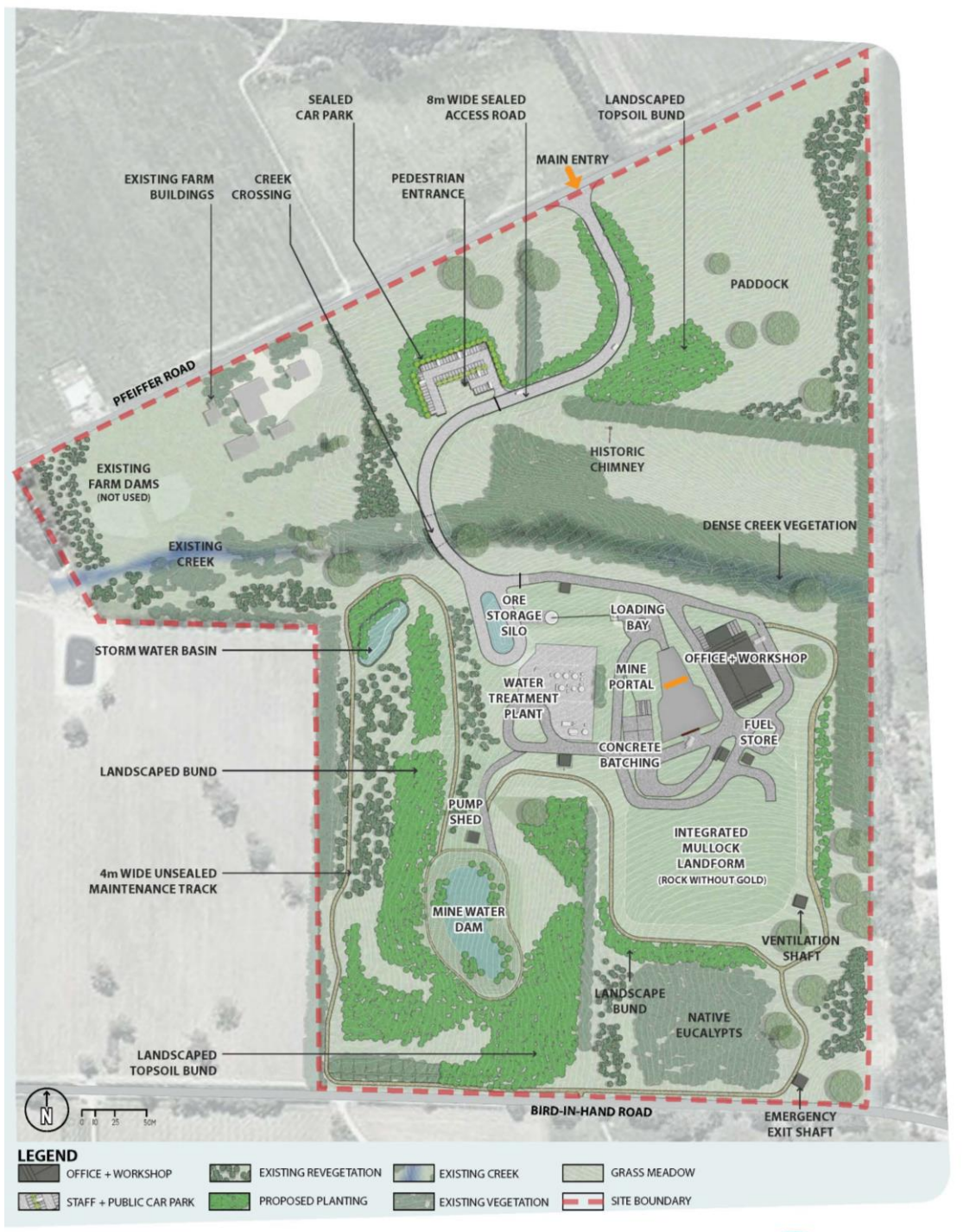
FIGURE 2-6 | SITE PLAN OF SURFACE INFRASTRUCTURE PROPOSED ON GOLDWYN
