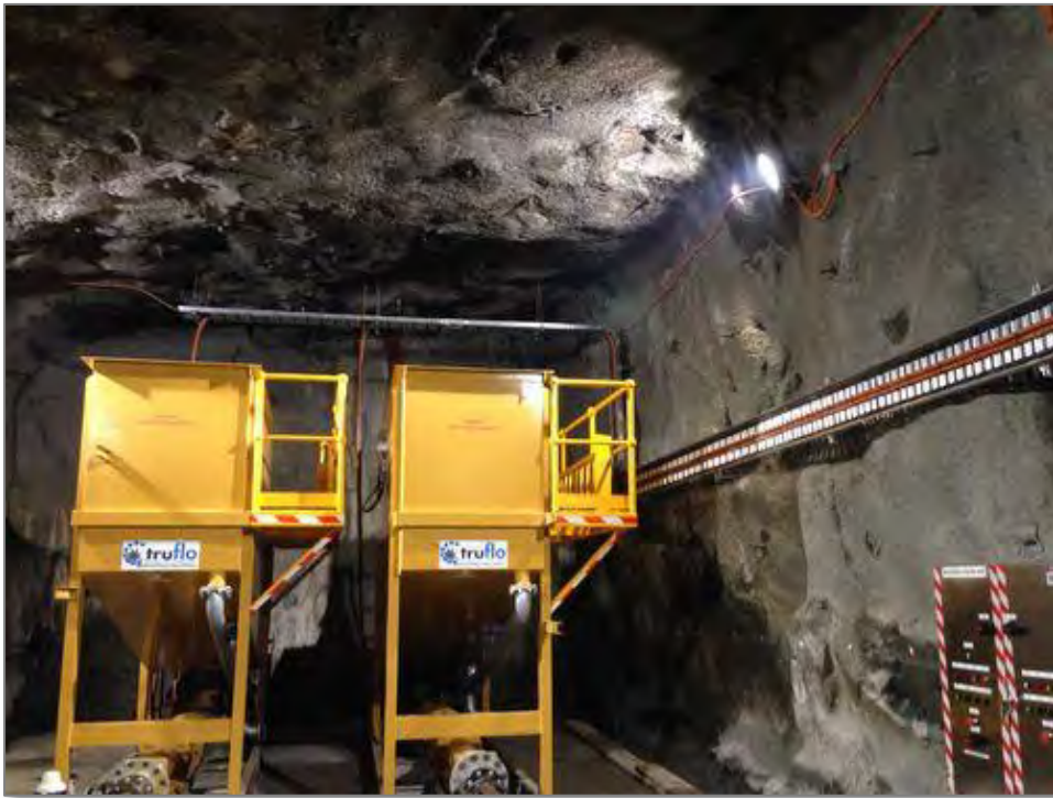
FIGURE 3-96 | TYPICAL MONO TYPE PUMP SET UP FOR UNDERGROUND GROUNDWATER MANAGEMENT. (COMPLIANCE ELECTRICAL, 2017)
