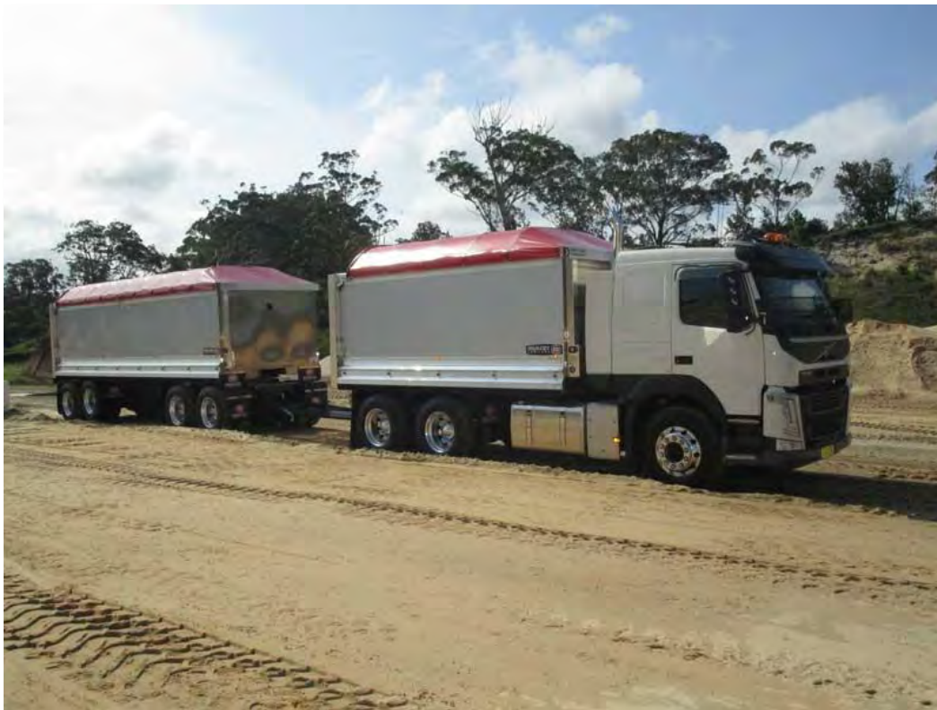
FIGURE 3-108 | ORE HAULAGE VEHICLE PROPOSED - 19M RIGID TRUCK AND DOG COMBINATION WITH COVERED LOAD
