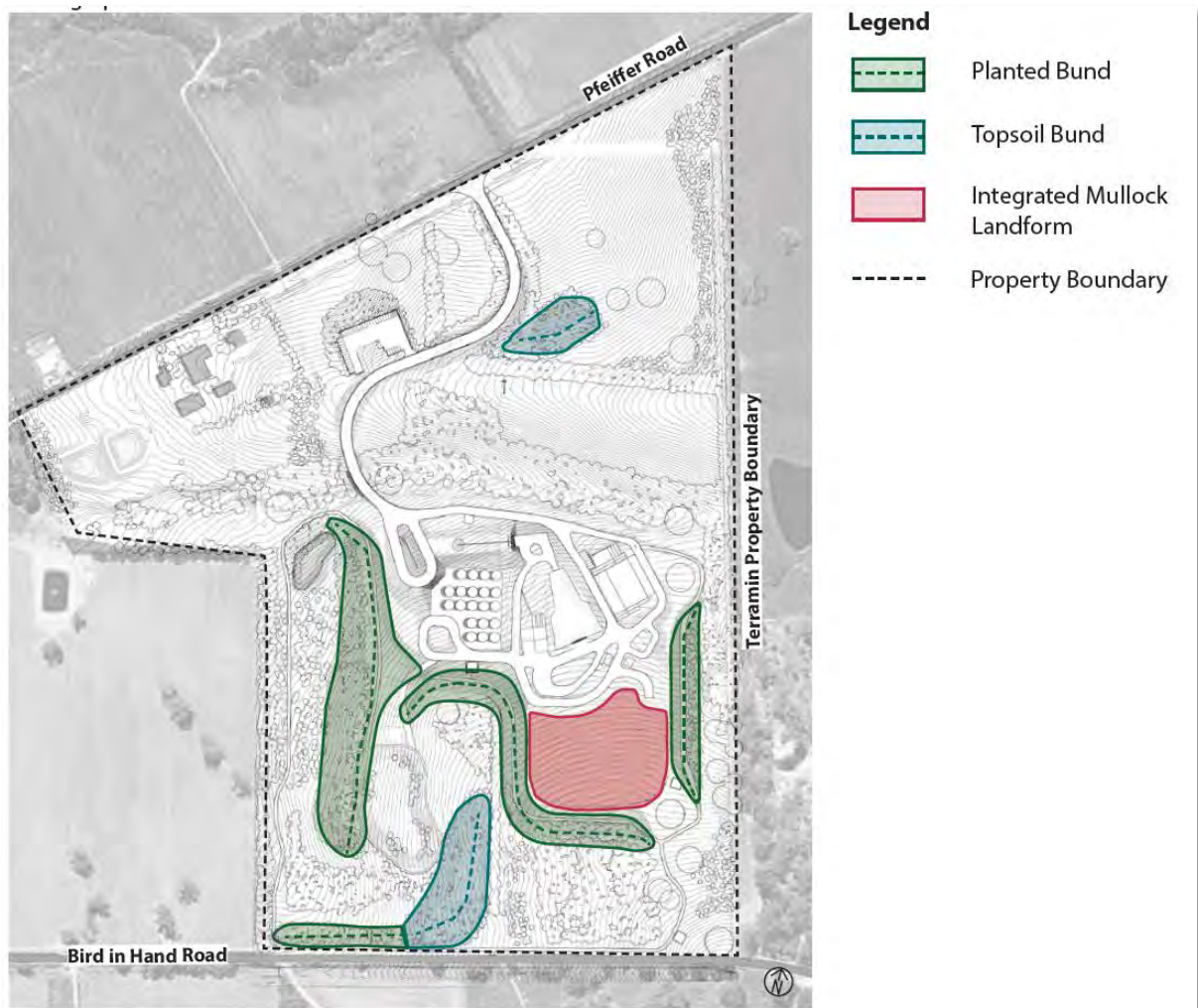
FIGURE 3-151 | PLANNED EARTH BUNDING TO ASSIST WITH VISUAL SCREENING OF SITE INFRASTRUCTURE (APPENDIX G1)
