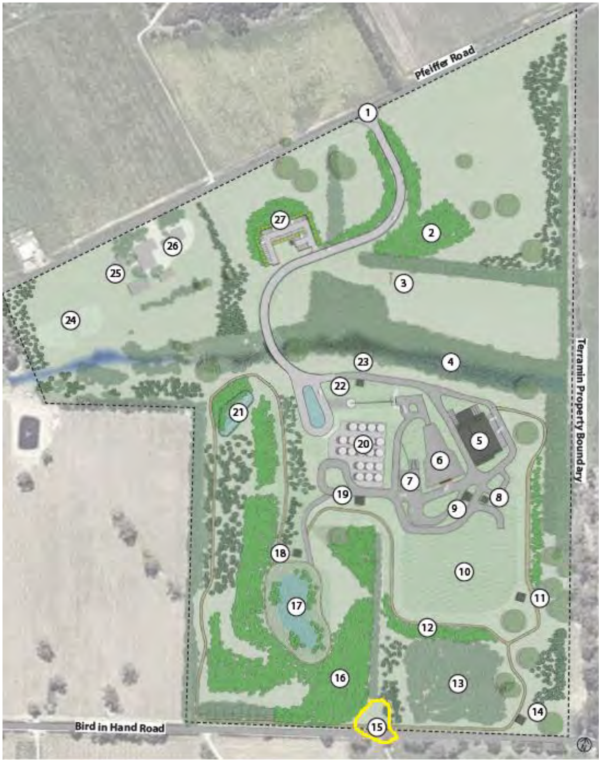
FIGURE 3-144 | CONCEPTUAL SITE DESIGN SHOWING EMERGENCY ACCESS POINT FROM BIRD-IN-HAND ROAD (APPENDIX G1)
