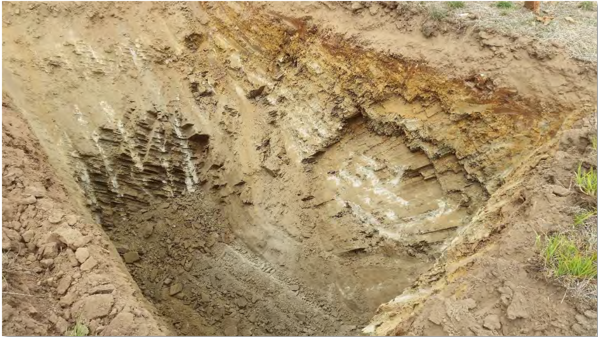
FIGURE 3-28 | PHOTO OF ONE OF THE GEOTECHNICAL TEST PITS USED BY MINING ONE TO IDENTIFY THE ROCK PROPERTIES USED TO DESIGN THE BOXCUT AND PORTAL LOCATION
