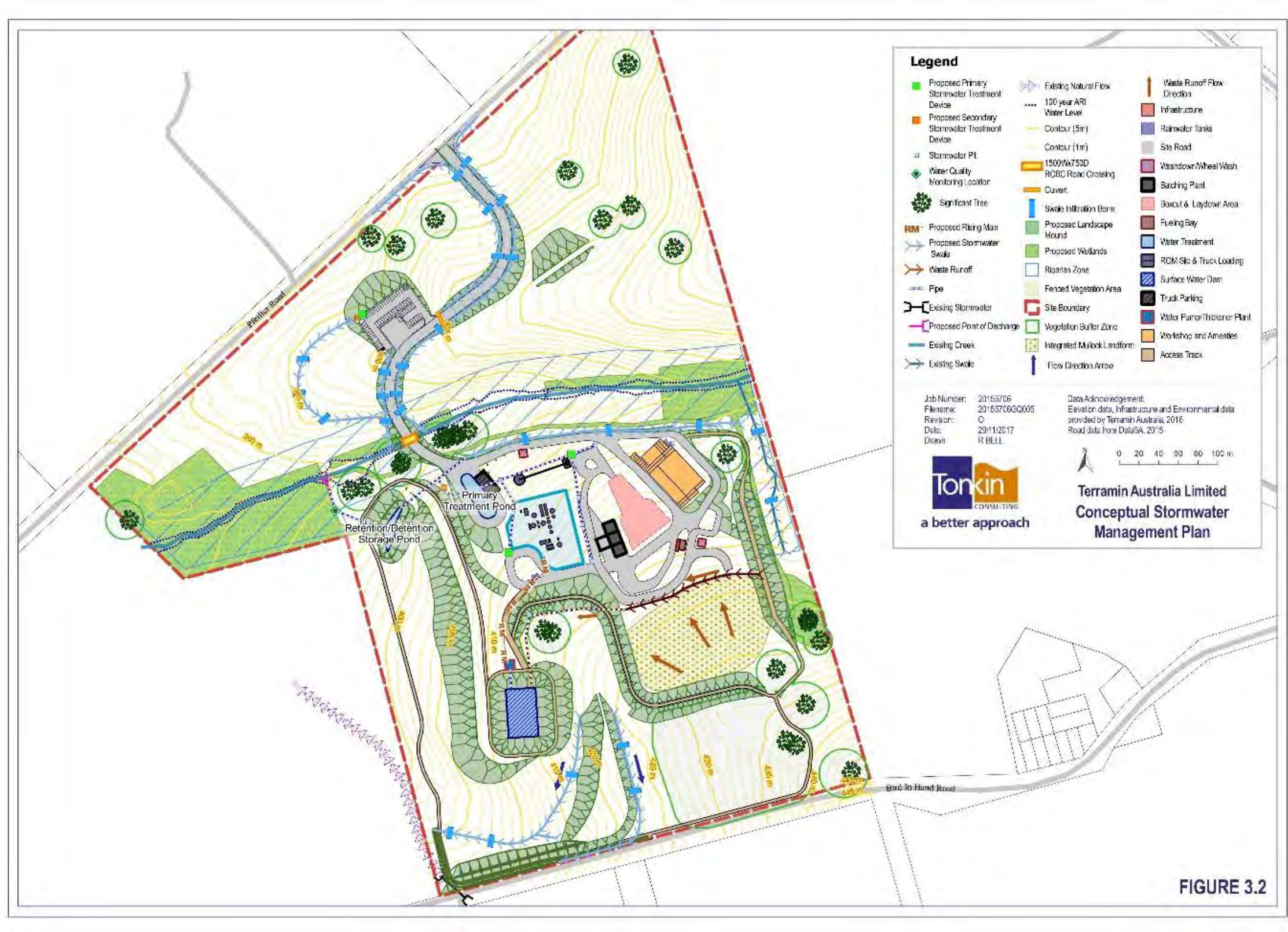
FIGURE 3-130 | STORMWATER MANAGEMENT PLAN SHOWING SURFACE RUN-OFF FROM THE IML BEING DIRECTED TO THE SURFACE WATER DAM (APPENDIX I3)
