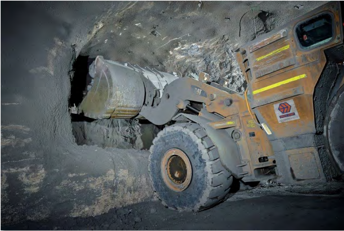
FIGURE 3-114 | UNDERGROUND LOADER TIPPING MATERIAL INTO AN UNDERGROUND ORE/WASTE PASS (INDUSTRY QUEENSLAND, 2016)
