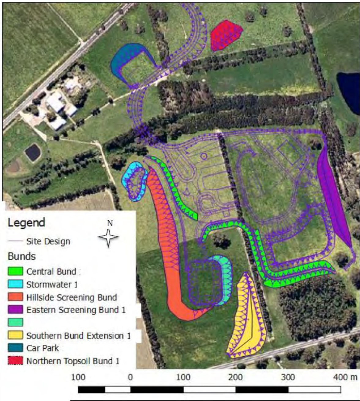
FIGURE 3-129 | BIH SITE DESIGN WITH THE PROPOSED BUNDS WHICH HAVE THE POTENTIAL FOR EROSION (APPENDIX L5)
