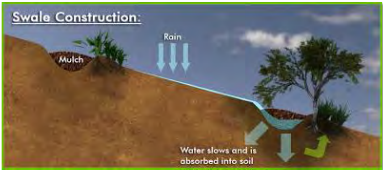
FIGURE 3-178 | EXAMPLE OF TYPICAL SWALE CONSTRUCTION ON A SLOPE FOR STORM WATER MANAGEMENT (TEMPERATE CLIMATE PERMACULTURE, 2011)
