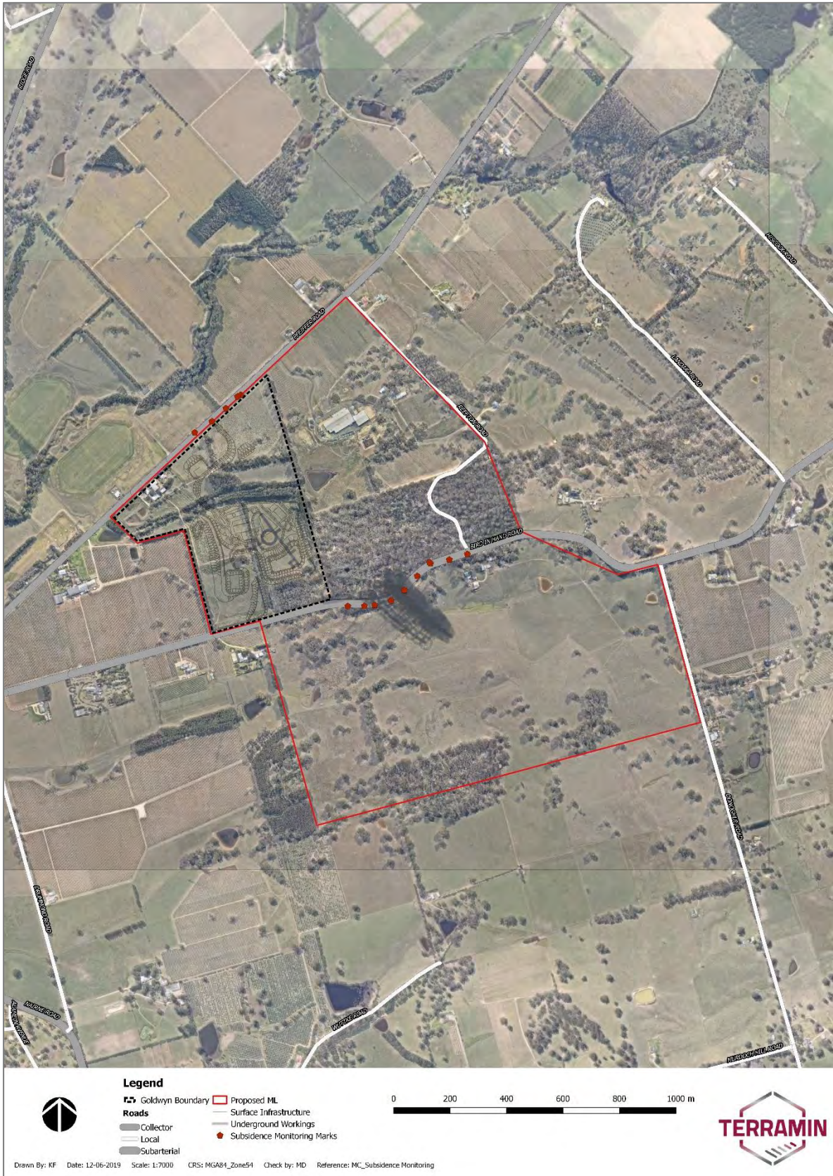
FIGURE 3-37 | LOCATION OF SUBSIDENCE MONITORING POINTS RELATIVE TO PROPOSED UNDERGROUND AND SURFACE EXCAVATION
