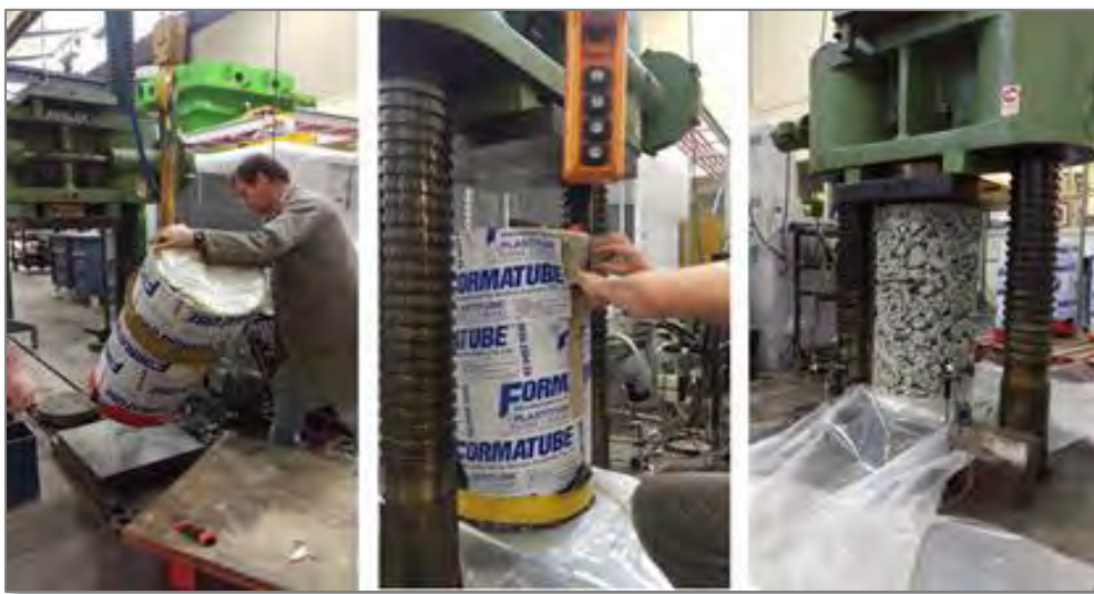
FIGURE 3-53 | FORMATUBE CRF CYLINDERS AND UCS TESTING APPARATUS AT MONASH UNIVERSITY (SAINSBURY, 2016)
