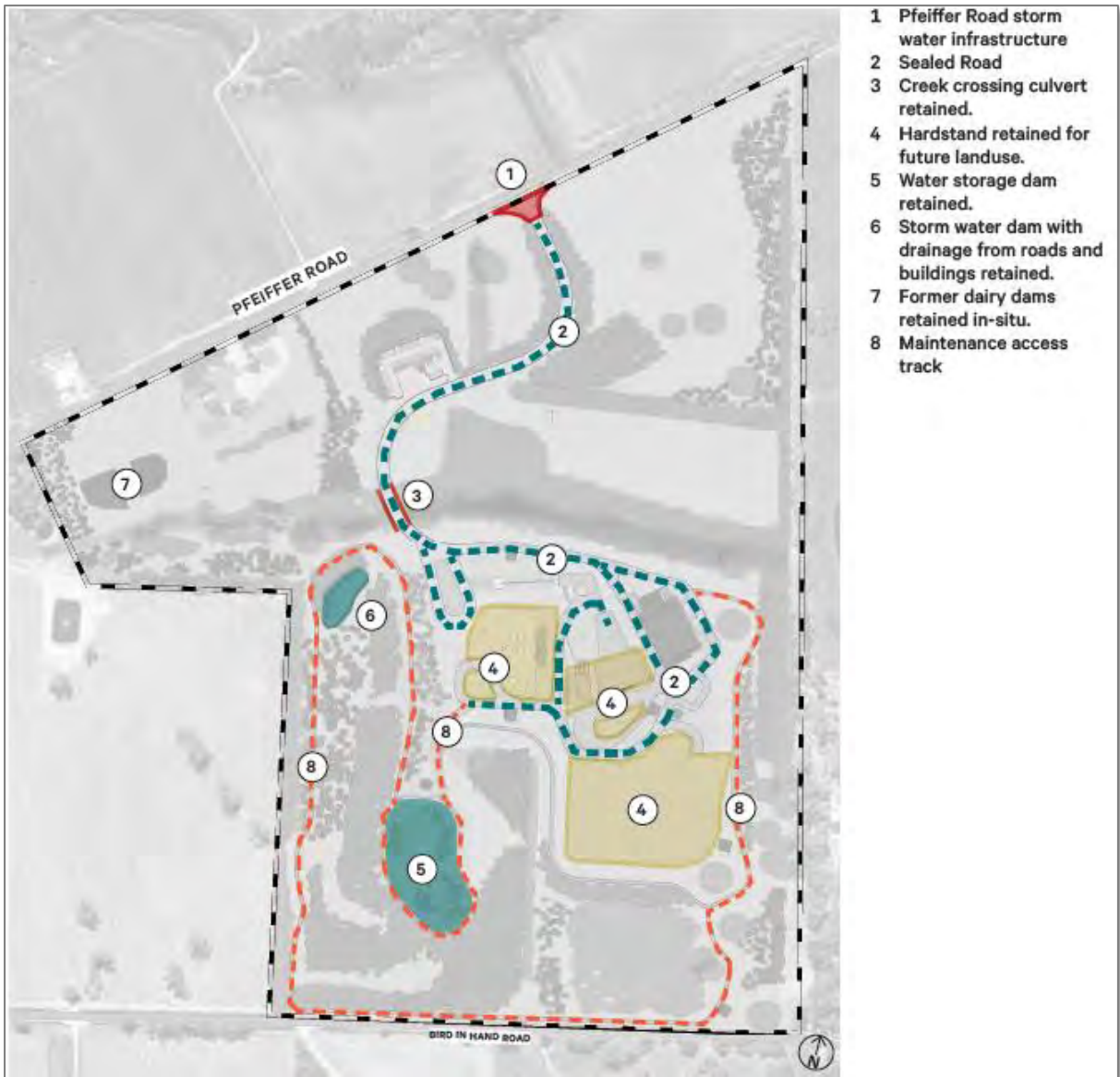
FIGURE 3-214 | INFRASTRUCTURE AND HARDSTAND REMAINING AT MINE COMPLETION (APPENDIX X1)
