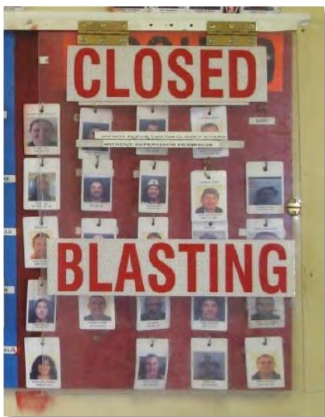
FIGURE 3-166 | EXAMPLE OF A TAG BOARD USED FOR UNDERGROUND MINING OPERATIONS
