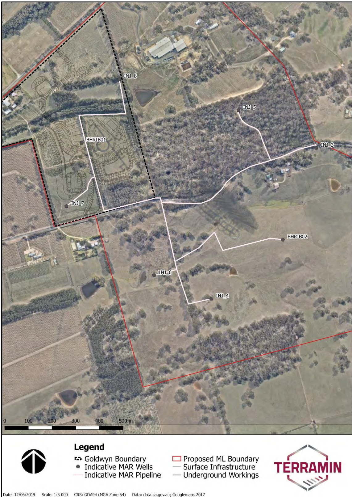
FIGURE 3-112 | PROPOSED MAR BORE LOCATIONS AND ASSOCIATED PIPELINES
